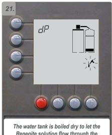
The water tank is boiled dry to let the Renegite solution flow through the circulation element.
