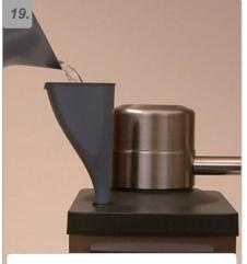
Place the funnel in the filling opening. Carefully pour the Renegite solution through the funnel.
