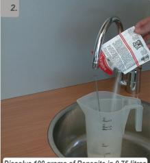
Dissolve 100 grams of Renegite in 0.75 litres of hand-warm water (approx. 40 °C). Stir the descaling solution, so that the agent is solved well.
